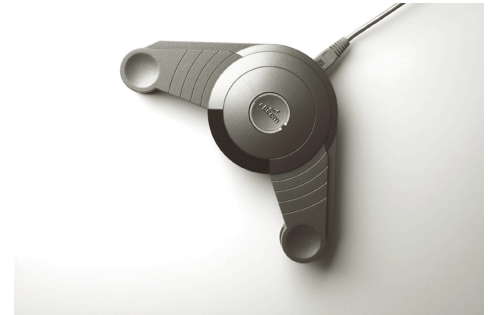
The eBeam capture unit, attached to the corner of the whiteboard.
